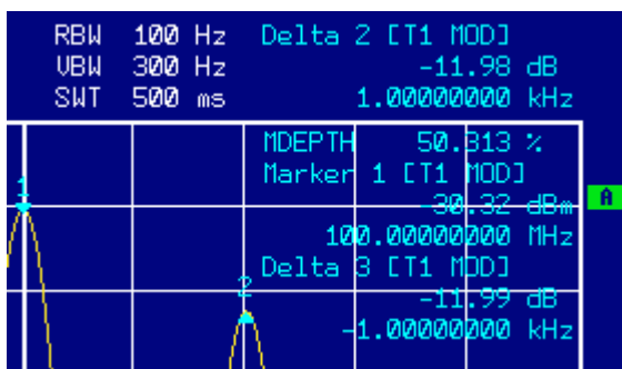
Fig. 5-7 Measurement of the AM modulation depth. The modulation depth shown is MDEPTH. The frequency of the AF signal can be obtained from the frequency display of the delta marker.
